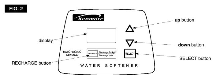
When the transformer is plugged in, a model code, and a test number (example: S3.0) show in the face plate display for 4 seconds. Then, 12:00 AM and PRESENT TIME begin to flash.
